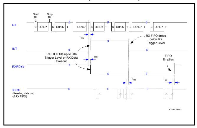
FIGURE 24. TRANSMIT READY & INTERRUPT TIMING [FIFO MODE, DMA MODE DISABLED] FOR CHANNELS A-D
