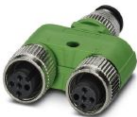
Y distributor, 4-position, unshielded, Plug straight M12, coding: A, on Socket straight M12, coding: A and Socket straight M12, coding: A
