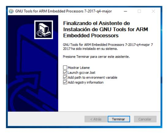
Once it is installed in your system you should be able to execute it by running the arm-noneeabi-gcc.exe --version command from a command line, i.e. Windows PowerShell. If the installation was successful you should see a terminal like the next image.
