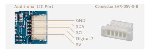
If you are interested in designing your own modules for Arduino boards with this expansion port, the connector we suggest using is code: SHR-05V-S-B, also in the picture.
