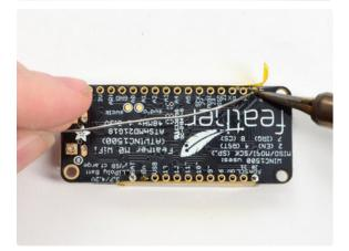
Flip & Tack Solder After flipping over, solder one or two points on each strip, to 'tack' the header in place
