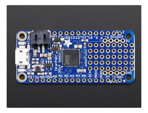
At the Feather 32u4's heart is at ATmega32u4 clocked at 8 MHz and at 3.3V logic, a chip setup we've had tons of experience with as <u>it's the same as the Flora</u> (https://adafru.it/dVI). This chip has 32K of flash and 2K of RAM, with built in USB so not only does it have a USB-to-Serial program & debug capability built in with no need for an FTDI-like chip, it can also act like a mouse, keyboard, USB MIDI device, etc.
