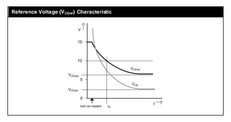
After  $t_{bl}$  has passed, the  $V_{CE}$  monitoring will be triggered as soon as  $V_{CE} > V_{CEref}$  and will turn off the IGBT. The error memory will be set, and the output PRIM\_nERROR\_OUT changes to the HIGH state. Possible failure modes are shows in the following pictures.
