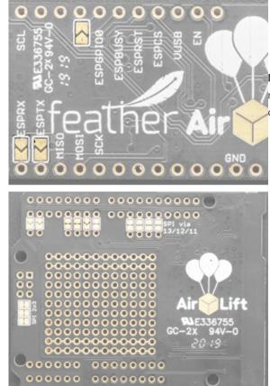
Make sure to solder each of these pads together. You will not be able to upload firmware to your ESP32 if they are not connected.
