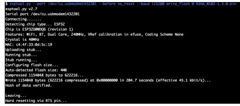
Once the firmware is fully uploaded, the ESP32 will reset.
