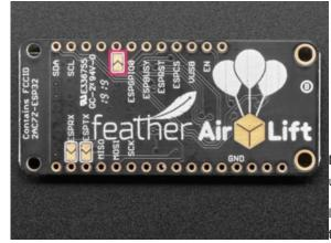
Note: These pin definitions leave the the ESP32's GPIOO pin undefined (-1).
