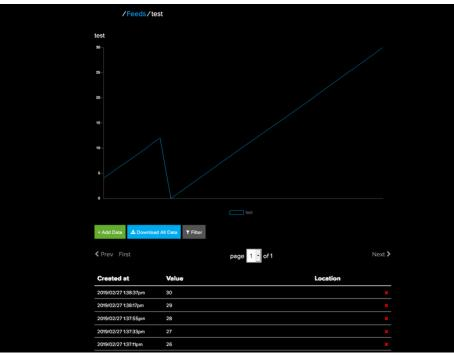
We can then have a simple loop for posting data to Adafruit IO without having to deal with connecting or initializing the hardware!
