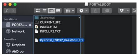
The lights should flash again, **BOOT** will disappear. Your board should re-enumerate USB and appear as a COM or Serial port on your computer. Make a note of the serial port by checking the **Device Manager** (Windows) or **typing Is /dev/cu\* or /dev/tty\*** (Mac or Linux) **in a terminal.**
