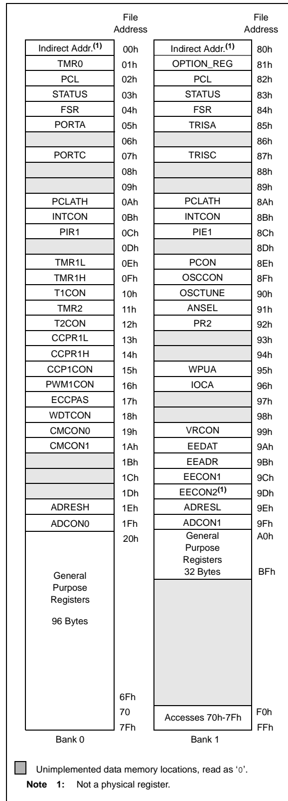
FIGURE 2-2: DATA MEMORY MAP OF THE PIC16F684
