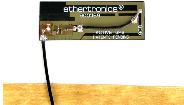
Antenna is stuck to a piece of plastic made of ABS
