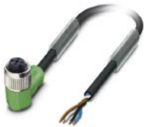
Sensor/actuator cable, 4-position, PUR halogen-free, black-gray RAL 7021, free cable end, on Socket angled M12, coding: A, cable length: 5 m
