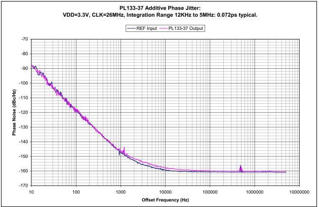
FIGURE 1-1: PL133-37 Additive Phase Jitter.
