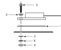
Note: Smooth side of flat washer should be placed against insulator when using the kit.
