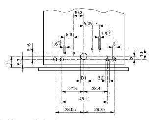
Fixation on PCB or housing from below
