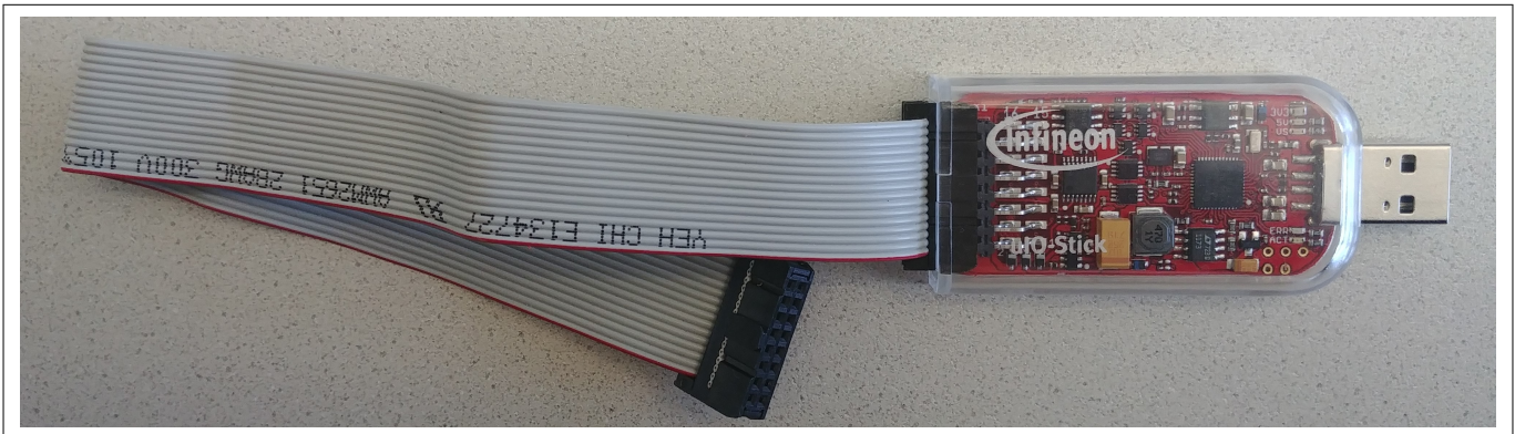
Figure 11 Infineon \mu IO-Stick with ribbon cable
