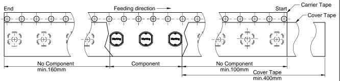
detail B Cover Tape Chip Cavity Sprocket Hole
