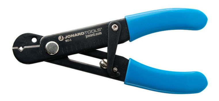
Designed with a precision-ground "V" notch blade and adjustable blade stop for superior stripping, this adjustable wire stripper and cutter is perfect for stripping and cutting 10-30 AWG (2.6-0.25 mm) solid and stranded wire. This stripper features the following:
