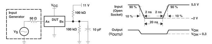
Figure 1. Device Test Setup
