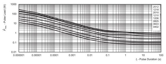
Maximum pulse load, continuous pulses; applicable if  $\overline{P} \leq P$  ( $\theta_{amb}$ ) and  $\hat{U} = \hat{U}_{max}$ ; for permissible resistance change equivalent to 8000 h operation
