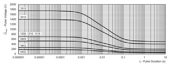
Maximum pulse voltage, single and continuous pulses; applicable if  $\hat{P} = \hat{P}_{max}$ ; for permissible resistance change equivalent to 8000 h operation
