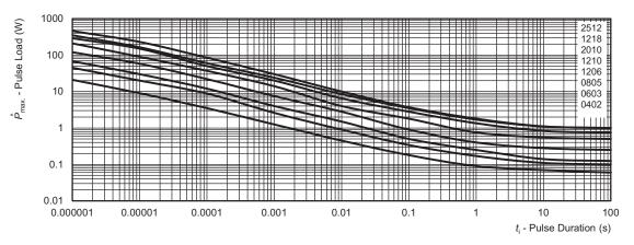
Maximum pulse load, single pulse; applicable if  $\overline{P} \rightarrow 0$  and n < 1000 and  $\hat{U} = \hat{U}_{max}$ ; for permissible resistance change equivalent to 8000 h operation
