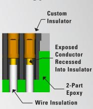
Cinch's unique plug insulators are designed to provide increased electrical protection between contact cavities preventing any potential shorts due to exposed wire or epoxy voids. Comprised of LCP material these connectors offer superior performance and long life in severe environments.
