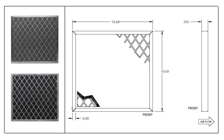
Orion Fans Hydrophobic Mesh air filters are water-repellent and offer a low pressure drop, cost-effective solution. The combination of hydrophobic mesh on the downstream side and high density foam on the upstream side offers a durable, cleanable, and moisture-resistant product. Designed for outdoor cabinets, process equipment applications requiring mist elimination, or other harsh environment installations.
