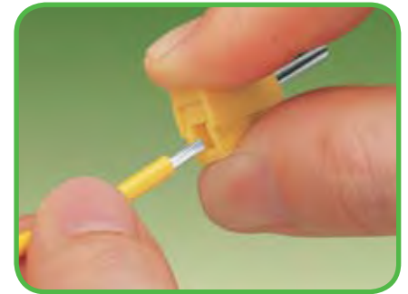
Connection of conductors: Press button fully and insert stripped conductor into square entry and release
