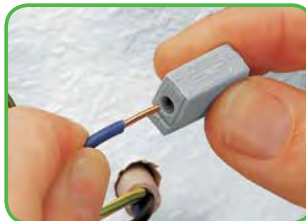
Connection of conductors (installation side): Introduce stripped solid conductor into circular entry and push to stop.
