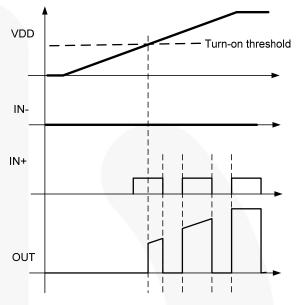
Figure 52. Non-Inverting Startup Waveforms
