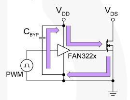
Figure 48. Current Path for MOSFET Turn-On
