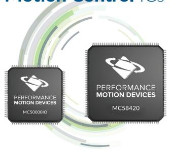
The Magellan Family of Motion Control ICs provide advanced motion control for medical, scientific, automation, industrial, and robotic applications. Available in 1, 2, 3, and 4-axis versions, these flexible, programmable devices control Brushless DC, DC Brush, and step motors.
