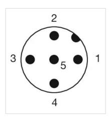
1 = Shield 2 = Red (AWG22) 3 = Black (AWG22) 4 = White (AWG24) 5 = Blue (AWG24)
