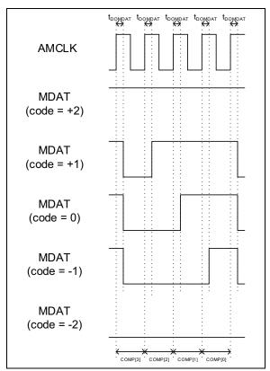
FIGURE 5-3:MDAT Serial OutputsDepending on the Modulator Output Code.
