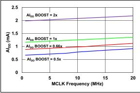
**FIGURE 2-56:**  $AI_{DD}$  vs MCLK (internal  $V_{REF}$ ).
