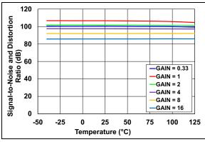
FIGURE 2-26: SINAD vs. Temperature, External V<sub>REF</sub>.
