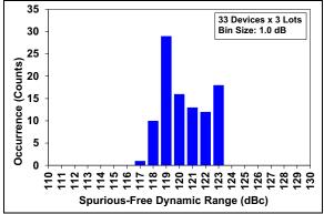
**FIGURE 2-21:** SFDR Distribution Histogram External V<sub>REF</sub>.
