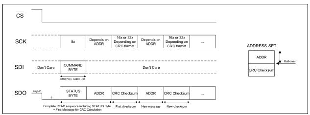
FIGURE 6-11: SPI Static Read with Communication CRC Enabled.
