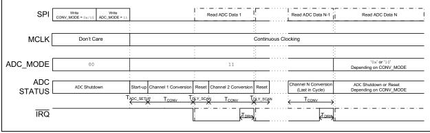
FIGURE 5-16: SCAN One-Shot Conversion Mode Timing Diagram.
