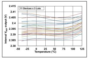
**FIGURE 2-59:**  $V_{REF}$  Output Voltage vs Temperature (AV<sub>DD</sub> = 3.3V).
