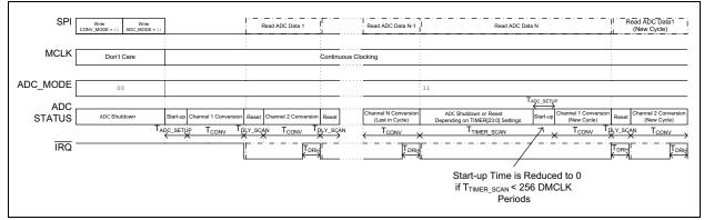
FIGURE 5-17: SCAN Continuous Conversion Mode Timing Diagram.
