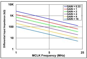
FIGURE 2-52: Differential Input Impedance vs. MCLK.
