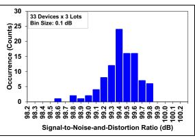
FIGURE 2-23: SINAD Distribution Histogram Internal V<sub>REF.</sub>
