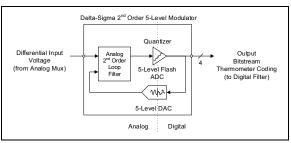
FIGURE 5-2: Simplified Delta-Sigma ADC Block Diagram.
