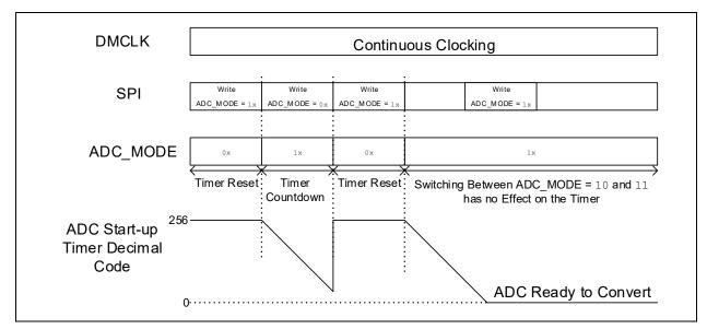
FIGURE 5-11: ADC Start-up Timer Timing Diagram.
