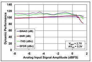
FIGURE 2-34: Dynamic Performance vs. Input Signal Amplitude.
