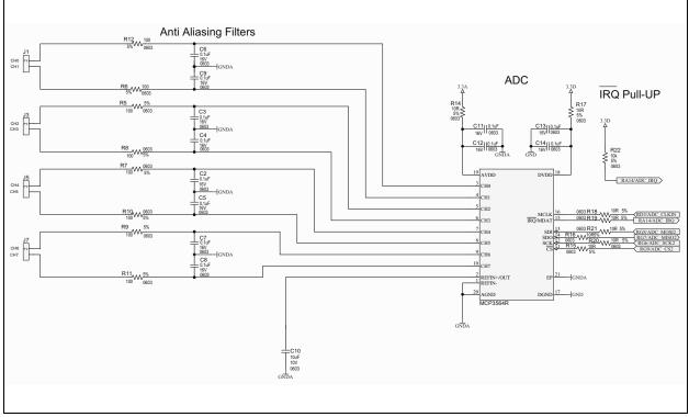
FIGURE 7-1: MCP3564R Application Example.
