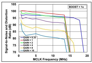
**FIGURE 2-41:** SINAD vs. AMCLK (BOOST = 1X, Internal  $V_{REF}$ ).
