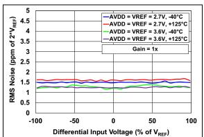
FIGURE 2-8: Output Noise vs. Input Voltage.
