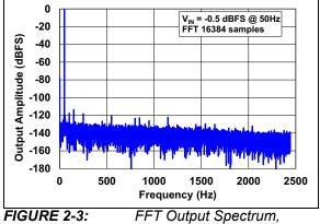
$f_{in} = 50 \text{ Hz} (Internal V_{REF}).$
