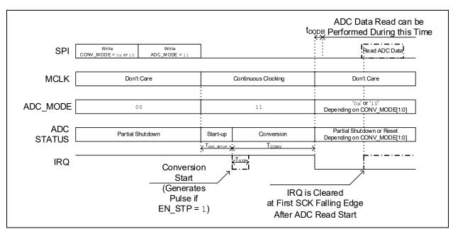
FIGURE 5-14: MUX One-Shot Conversion Mode Timing Diagram.
