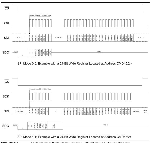
**FIGURE 6-4:** Single Register Write Communication (CMD[1:0] = 10) Timing Diagram.
