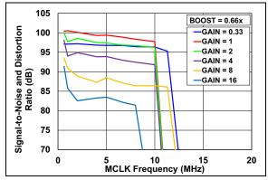
**FIGURE 2-40:** SINAD vs. AMCLK (BOOST = 0.66X, Internal V<sub>REF</sub>).
