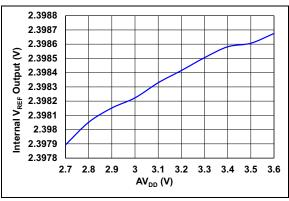
**FIGURE 2-60:** Internal V<sub>REF</sub> Output Voltage vs. AV<sub>DD.</sub>
