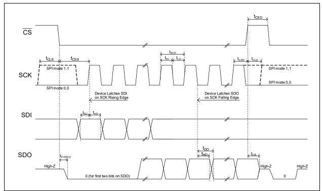
FIGURE 1-1: Serial Output Timing Diagram.
