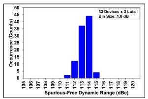
FIGURE 2-25: SFDR Distribution Histogram Internal V<sub>REF.</sub>
