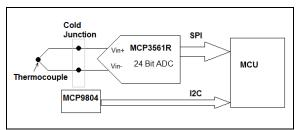
FIGURE 7-2: Thermocouple Connection to MCP3561R.
