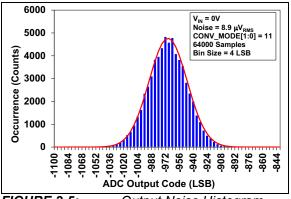
**FIGURE 2-5:** Output Noise Histogram (External V<sub>REF</sub>).
