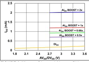
**FIGURE 2-55:**  $DI_{DD}$  and  $AI_{DD}$  vs.  $DV_{DD}$  and  $AV_{DD}$ .
