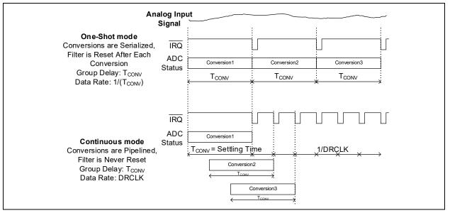
FIGURE 5-5: One-Shot Mode vs. Continuous Mode.
