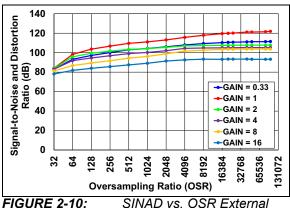
FIGURE 2-10: SINAD vs. OSR Externa V<sub>REF</sub>.
