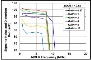
**FIGURE 2-39:** SINAD vs. AMCLK (BOOST = 0.5X, Internal V<sub>REF</sub>).
