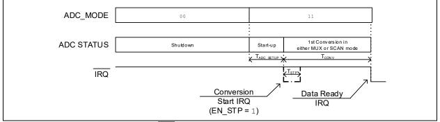
**FIGURE 6-14:** Conversion Start IRQ Timing Diagram.
