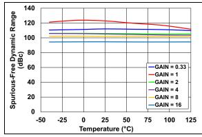
*FIGURE 2-29:* SFDR vs. Temperature, External V<sub>REF</sub>.
