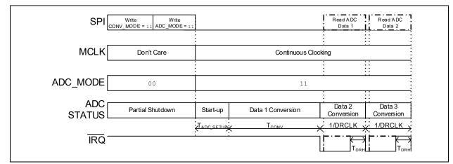
FIGURE 5-15: MUX Continuous Conversion Mode Timing Diagram.
