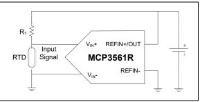
FIGURE 7-3: Wheatstone Bridge Ratiometric Connection.
