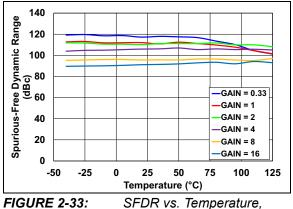
FIGURE 2-33: SFDR vs. Te Internal V<sub>REF.</sub>
