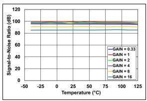
FIGURE 2-31: SNR vs. Temperature, Internal V<sub>REF.</sub>
