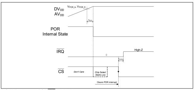
FIGURE 6-15: POR IRQ Timing Diagram.
