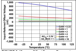
FIGURE 2-48: Offset Error vs. Temperature (AZ\_MUX = 1).
