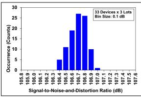
*FIGURE 2-19:* SINAD Distribution Histogram External V<sub>REF</sub>.
