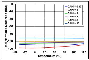
FIGURE 2-28: THD vs. Temperature, External V<sub>REF</sub>.
