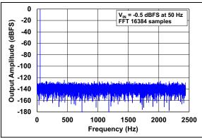
**FIGURE 2-1:** FFT Output Spectrum,  $f_{in} = 50$  Hz (External  $V_{REF}$ ).
