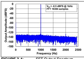
**FIGURE 2-4:** FFT Output Spectrum,  $f_{in} = 1 \text{ kHz}$  (Internal V<sub>REF</sub>).
