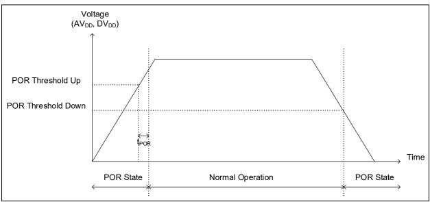
FIGURE 5-10: Power-on Reset Timing Diagram.
