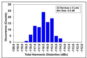
**FIGURE 2-20:** THD Distribution Histogram External V<sub>REF</sub>.
