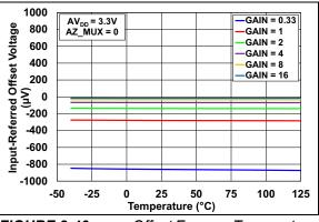
FIGURE 2-46: Offset Error vs. Temperature (AZ MUX = 0).
