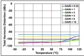
FIGURE 2-32: THD vs. Temperature, Internal V<sub>REF.</sub>
