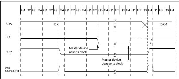
FIGURE 17-12: CLOCK SYNCHRONIZATION TIMING
