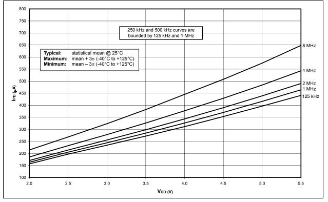
FIGURE 27-19: MAXIMUM IPD vs. VDD (-40°C TO +125°C), 125 kHz TO 8 MHz RC\_IDLE, ALL PERIPHERALS DISABLED
