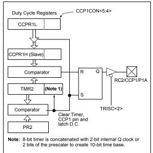
A PWM output (Figure 15-4) has a time base (*period*) and a time that the output is high (*duty cycle*). The frequency of the PWM is the inverse of the period (1/period).
