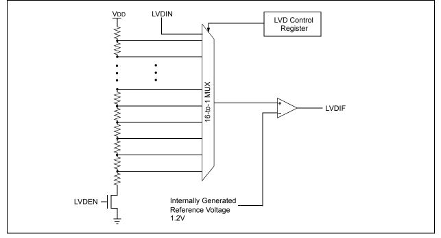
The LVD module has an additional feature that allows the user to supply the sense voltage to the module from an external source. This mode is enabled when bits LVDL3:LVDL0 are set to '1111'. In this state, the comparator input is multiplexed from the external input pin, LVDIN (Figure 22-3). This gives users flexibility because it allows them to configure the Low-Voltage Detect interrupt to occur at any voltage in the valid operating range.
