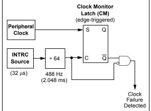
Clock failure is tested on the falling edge of the sample clock. If a sample clock falling edge occurs while CM is still set, a clock failure has been detected (Figure 23-4). This causes the following:
