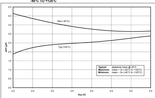
FIGURE 27-29: △IPD FSCM vs. VDD OVER TEMPERATURE PRI\_IDLE, EC OSCILLATOR AT 32 kHz, -40°C TO +125°C
