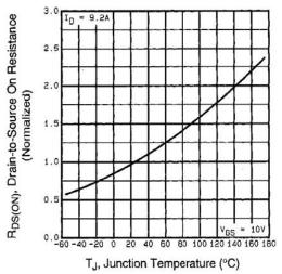
Fig. 4 - Normalized On-Resistance vs. Temperature
