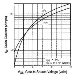
Fig. 3 - Typical Transfer Characteristics
