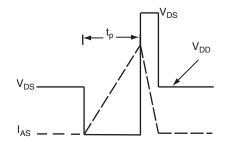
Fig. 12b - Unclamped Inductive Waveforms
