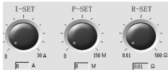
Fig.2-7 Current, Power, Resistance setting dial
