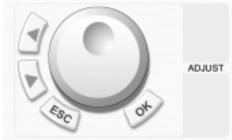
Fig.1-5 Rotary knob and function keys
