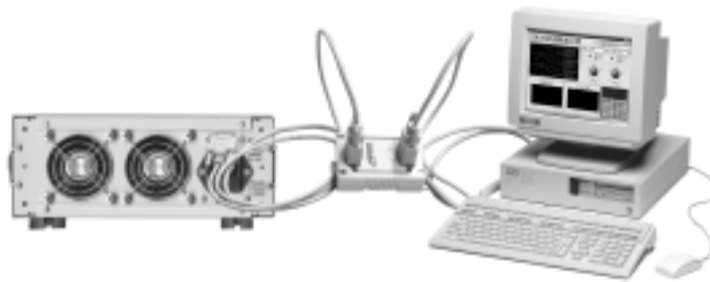
Fig.1-1 Connect the electronic load to PC
