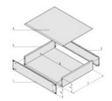
h = clear overall height (H - 3.0),b = clear installation width = 447 mm
