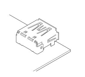
This connector is an interface connector conforming to USB (Universal Serial Bus) 3.0 Standard.
