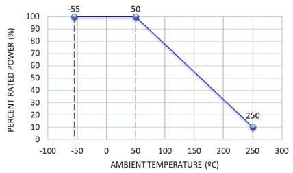
Note: This curve assumes the part is mounted on a properly sized heat sink.
