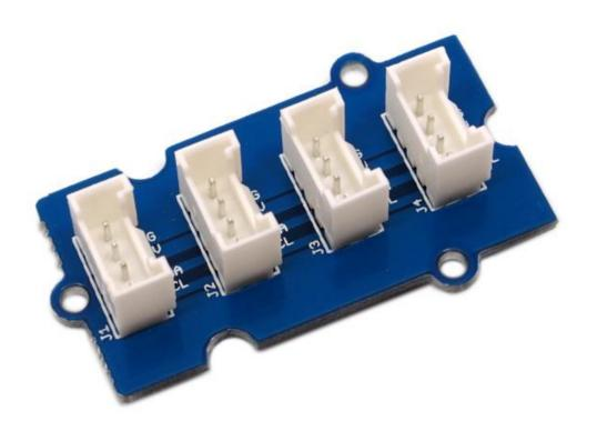
I2C Hub Grove is an extension Grove module for connecting multiply I2C devices to Grove Base Shield. It can use with Universal 4 Pin to X2 4 Pin cable and connects up to 3 I2C devices which may cover most developing purpose.
