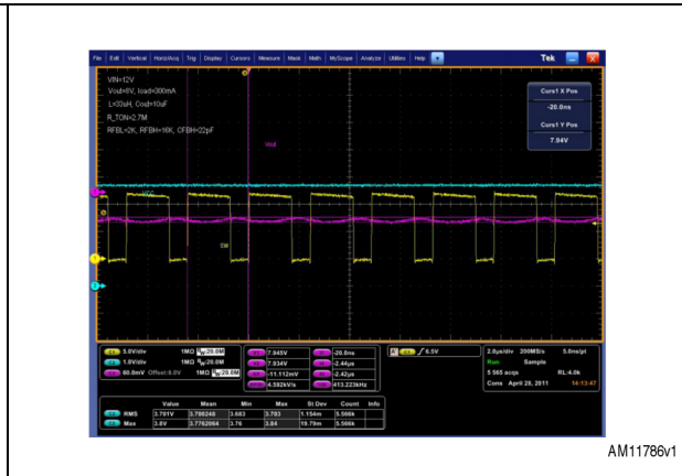
Figure 27. Load = 300 mA. Switching frequency = 410 kHz
