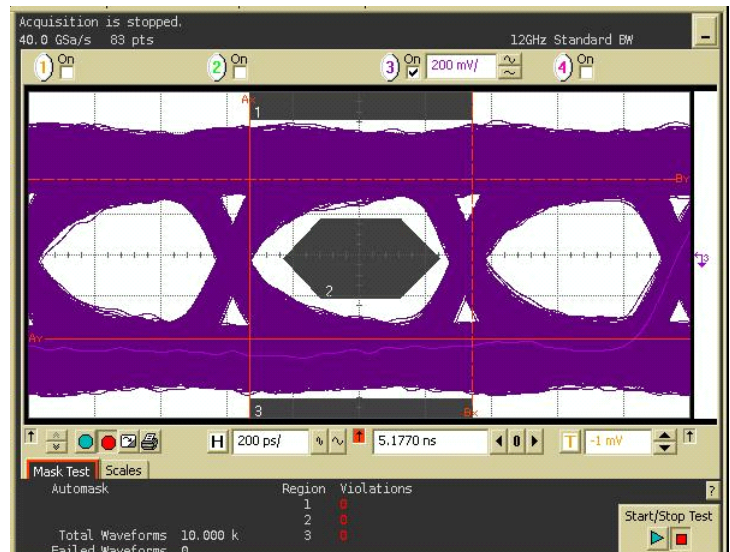
Figure 3 - Typical HDMI 1.3 Eye Pattern (1080p) with RClamp0524PA
