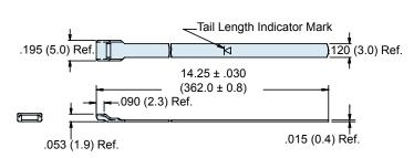
precision constructed of 300 Series SST/Passivate I.A.W. AMS 2700, and designed for use with the 600-061 Hand Banding Tool or the 600-068 Pneumatic Banding Tool. Double-wrapped bands will accommodate diameters up to approximately
