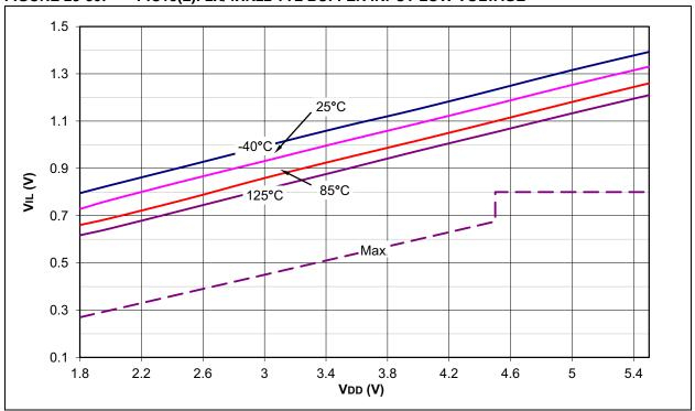
FIGURE 28-81: PIC18(L)F2X/4XK22 SCHMITT TRIGGER BUFFER INPUT LOW VOLTAGE
