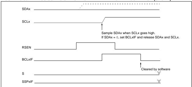
FIGURE 15-37: BUS COLLISION DURING REPEATED START CONDITION (CASE 2)
