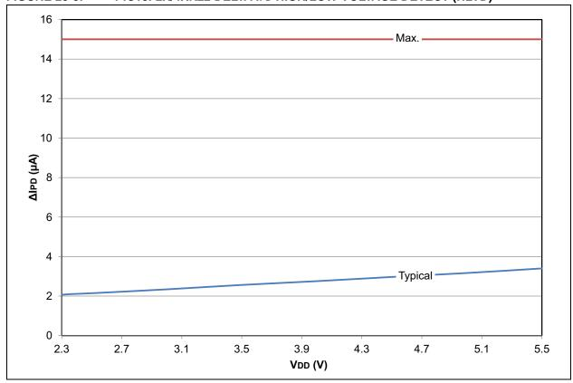
FIGURE 28-9: PIC18LF2X/4XK22 DELTA IPD SECONDARY OSCILLATOR
