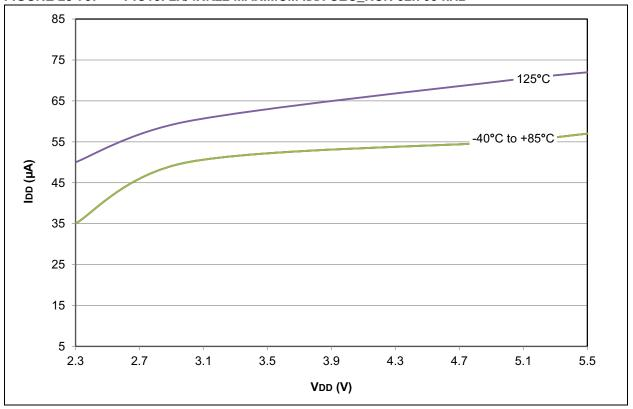
FIGURE 28-76: PIC18LF2X/4XK22 TYPICAL IDD: SEC\_IDLE 32.768 kHz
