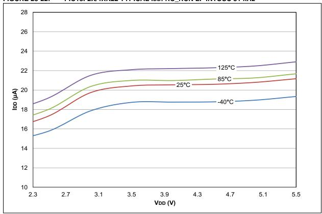
FIGURE 28-23: PIC18F2X/4XK22 MAXIMUM IDD: RC\_RUN LF-INTOSC 31 kHz
