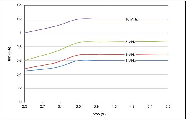
FIGURE 28-44: PIC18LF2X/4XK22 TYPICAL IDD: RC\_IDLE HF-INTOSC with PLL
