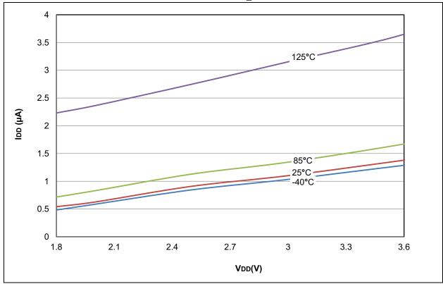
FIGURE 28-35: PIC18LF2X/4XK22 MAXIMUM IDD: RC\_IDLE LF-INTOSC 31 kHz
