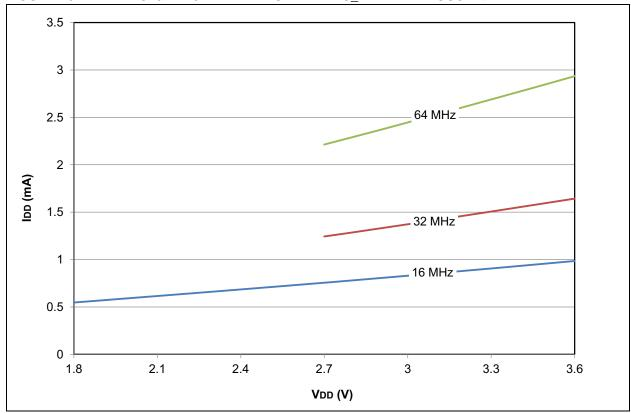
FIGURE 28-45: PIC18LF2X/4XK22 MAXIMUM IDD: RC\_IDLE HF-INTOSC with PLL
