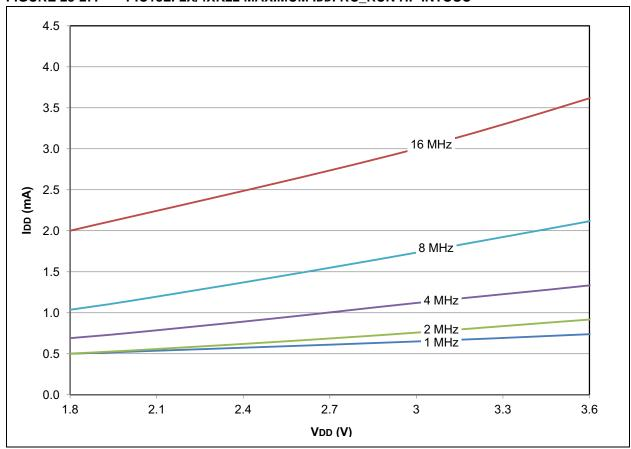
FIGURE 28-28: PIC18F2X/4XK22 TYPICAL IDD: RC\_RUN HF-INTOSC
