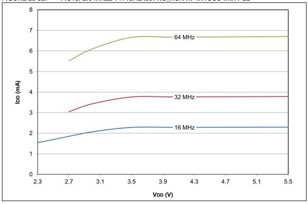
FIGURE 28-33: PIC18F2X/4XK22 MAXIMUM IDD: RC\_RUN HF-INTOSC with PLL
