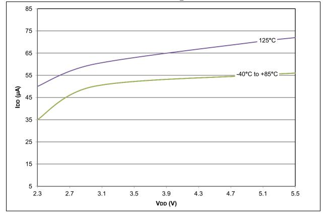
FIGURE 28-24: PIC18LF2X/4XK22 IDD: RC\_RUN MF-INTOSC 500 kHz
