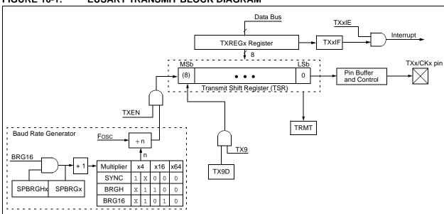
FIGURE 16-1: EUSART TRANSMIT BLOCK DIAGRAM
