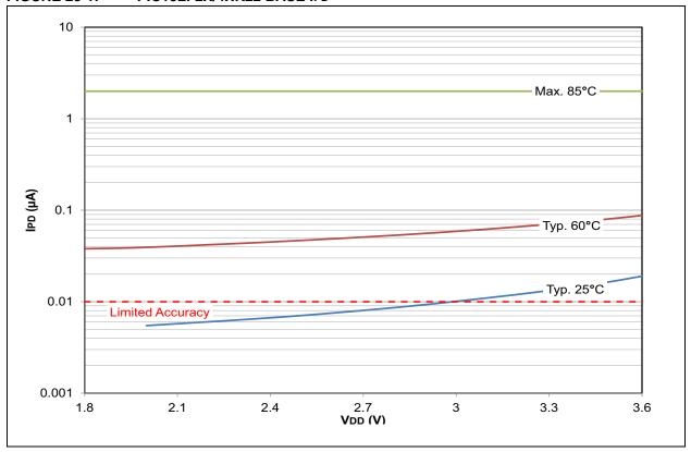
FIGURE 28-2: PIC18F2X/4XK22 BASE IPD
