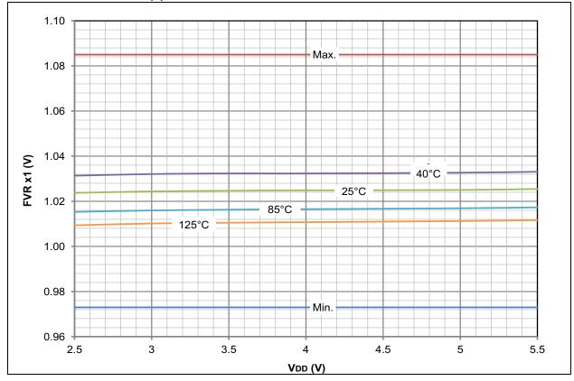
FIGURE 28-96: PIC18(L)F2X/4XK22 TYPICAL FIXED VOLTAGE REFERENCE 2x OUTPUT
