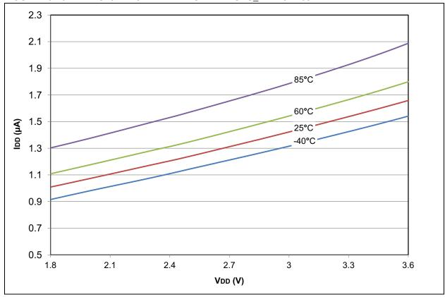
FIGURE 28-77: PIC18LF2X/4XK22 MAXIMUM IDD: SEC\_IDLE 32.768 kHz
