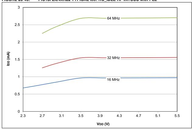
FIGURE 28-47: PIC18F2X/4XK22 MAXIMUM IDD: RC\_IDLE HF-INTOSC with PLL
