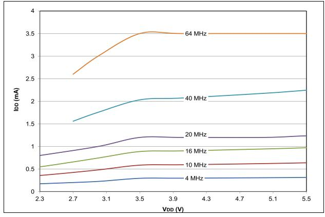
FIGURE 28-68: PIC18LF2X/4XK22 TYPICAL IDD: PRI\_IDLE EC with PLL
