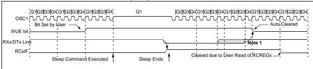
Note 1: If the wake-up event requires long oscillator warm-up time, the automatic clearing of the WUE bit can occur while the stposc signal is still active. This sequence should not depend on the presence of Q clocks.
