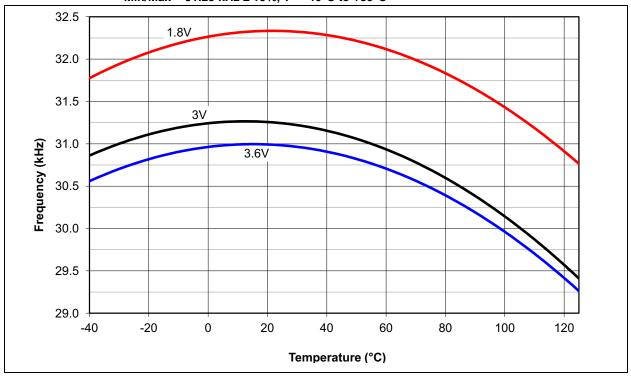
FIGURE 28-104: PIC18F2X/4XK22 TYPICAL LF-INTOSC FREQUENCY vs. TEMPERATURE Min/Max = 31.25 kHz ± 15%, T = -40°C to +85°C
