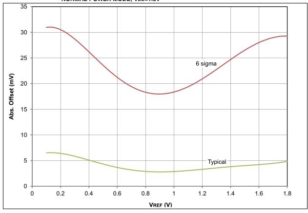
FIGURE 28-90: PIC18(L)F2X/4XK22 COMPARATOR OFFSET VOLTAGE, LOW-POWER MODE; VDD=5.5V
