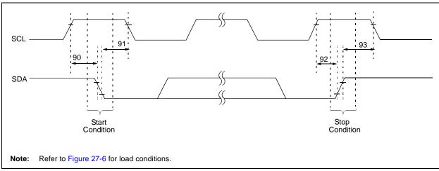
TABLE 27-15: I<sup>2</sup>C BUS START/STOP BITS REQUIREMENTS (SLAVE MODE)
