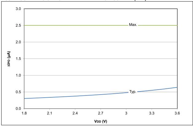
FIGURE 28-4: PIC18F2X/4XK22 DELTA IPD WATCHDOG TIMER (WDT)
