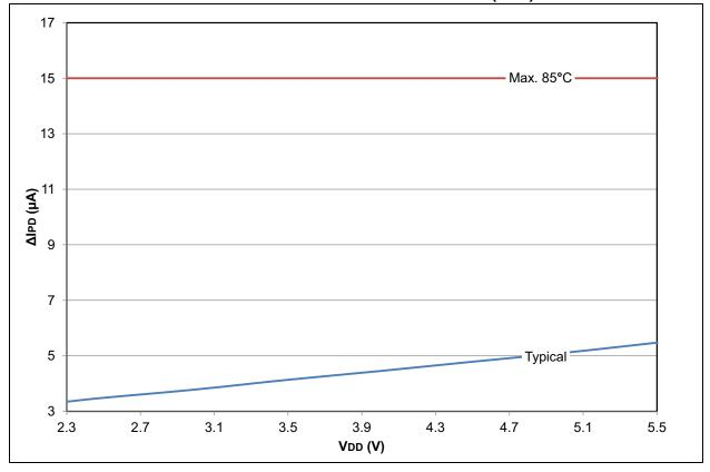
FIGURE 28-7: PIC18LF2X/4XK22 DELTA IPD HIGH/LOW-VOLTAGE DETECT (HLVD)
