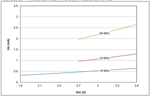
FIGURE 28-69: PIC18LF2X/4XK22 MAXIMUM IDD: PRI\_IDLE EC with PLL
