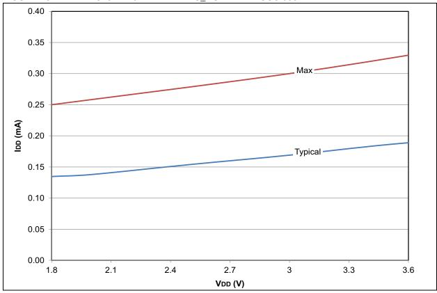
FIGURE 28-25: PIC18F2X/4XK22 IDD: RC\_RUN MF-INTOSC 500 kHz
