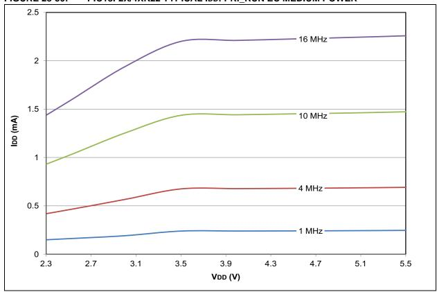
FIGURE 28-51: PIC18F2X/4XK22 MAXIMUM IDD: PRI\_RUN EC MEDIUM POWER
