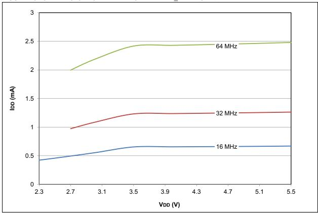
FIGURE 28-71: PIC18F2X/4XK22 MAXIMUM IDD: PRI\_IDLE EC with PLL
