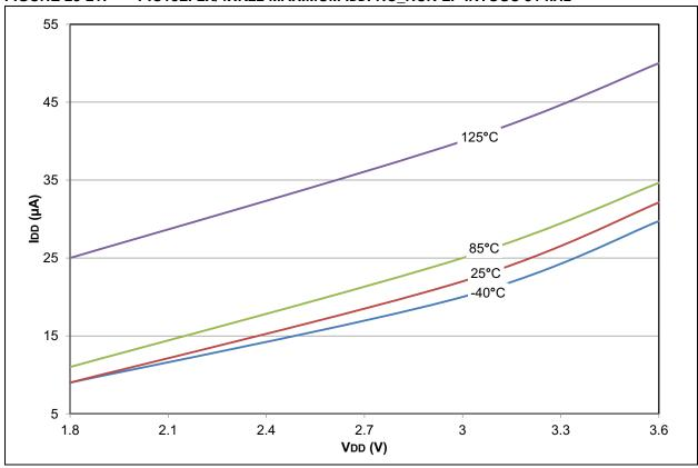
FIGURE 28-22: PIC18F2X/4XK22 TYPICAL IDD: RC\_RUN LF-INTOSC 31 kHz
