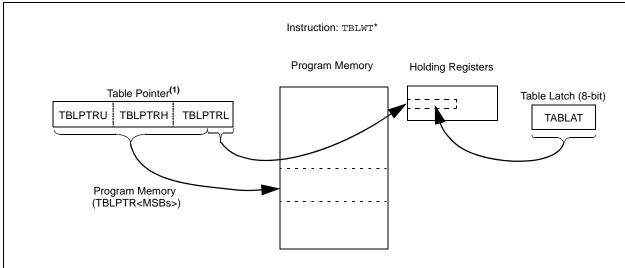
Note 1: During table writes the Table Pointer does not point directly to Program Memory. The LSBs of TBLPRTL actually point to an address within the write block holding registers. The MSBs of the Table Pointer determine where the write block will eventually be written. The process for writing the holding registers to the program memory array is discussed in Section 6.6 "Writing to Flash Program Memory".
