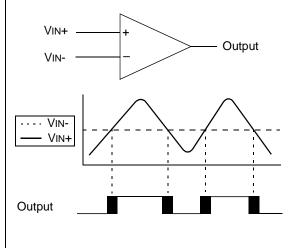
**Note:** The black areas of the output of the comparator represents the uncertainty due to input offsets and response time.
