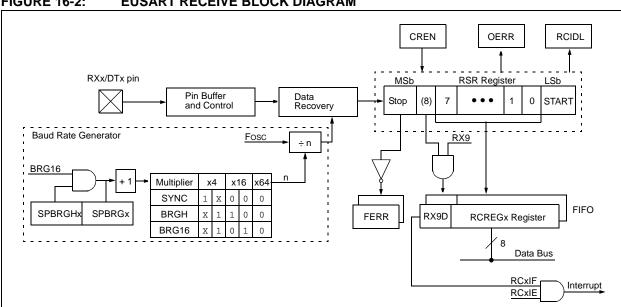
**FIGURE 16-2: EUSART RECEIVE BLOCK DIAGRAM**
