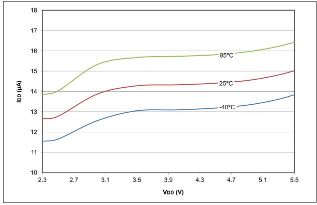
FIGURE 28-79: PIC18F2X/4XK22 MAXIMUM IDD: SEC\_IDLE 32.768 kHz
