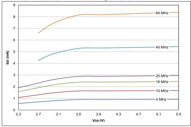
FIGURE 28-55: PIC18F2X/4XK22 MAXIMUM IDD: PRI\_RUN EC HIGH POWER
