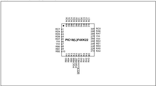
FIGURE 5: 44-PIN TQFP DIAGRAM
