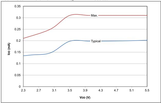
FIGURE 28-40: PIC18LF2X/4XK22 TYPICAL IDD: RC\_IDLE HF-INTOSC
