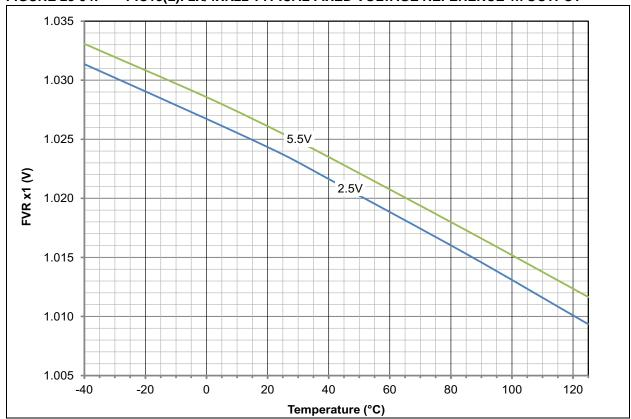
FIGURE 28-95: PIC18(L)F2X/4XK22 TYPICAL FIXED VOLTAGE REFERENCE 1x OUTPUT
