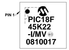
44-Lead QFN (8x8x0.9 mm)
