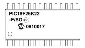
28-Lead SSOP (5.30 mm)
