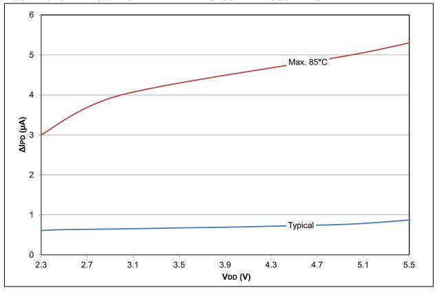
FIGURE 28-11: PIC18LF2X/4XK22 DELTA IPD COMPARATOR LOW-POWER MODE
