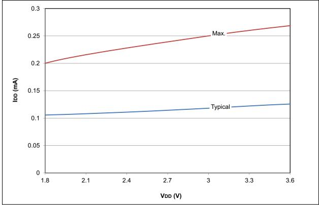
FIGURE 28-39: PIC18F2X/4XK22 IDD: RC\_IDLE MF-INTOSC 500 kHz
