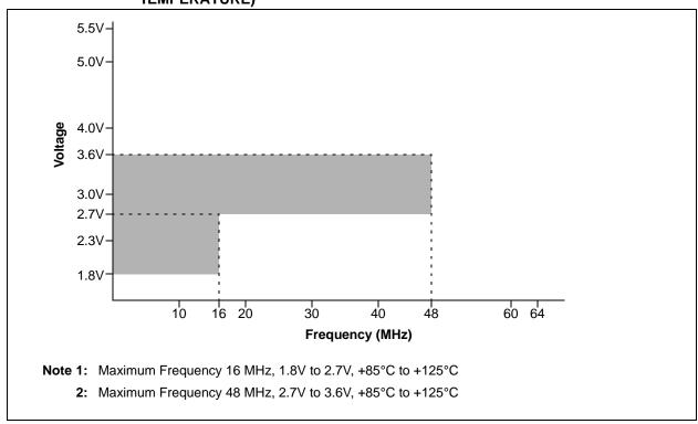
FIGURE 27-3: PIC18F2X/4XK22 FAMILY VOLTAGE-FREQUENCY GRAPH (INDUSTRIAL TEMPERATURE)
