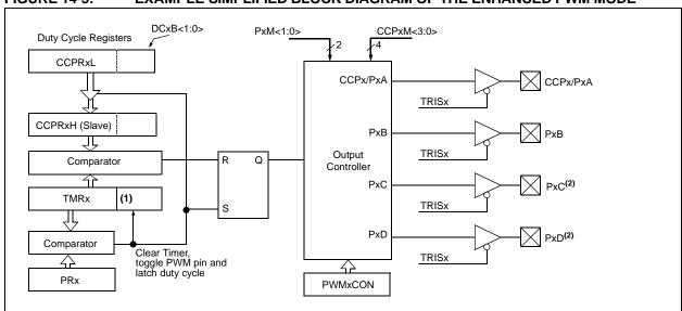
Note 1: The 8-bit timer TMRx register is concatenated with the 2-bit internal Q clock, or 2 bits of the prescaler to create the 10-bit time base.
