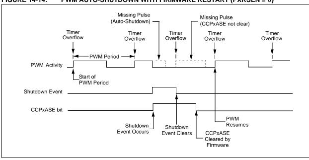
FIGURE 14-14: PWM AUTO-SHUTDOWN WITH FIRMWARE RESTART (PXRSEN = 0)
