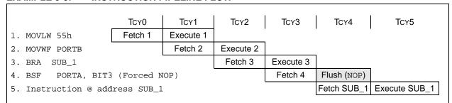
**Note:** All instructions are single cycle, except for any program branches. These take two cycles since the fetch instruction is "flushed" from the pipeline while the new instruction is being fetched and then executed.
