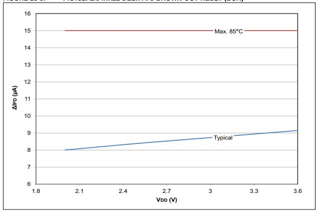
FIGURE 28-6: PIC18F2X/4XK22 DELTA IPD BROWN-OUT RESET (BOR)
