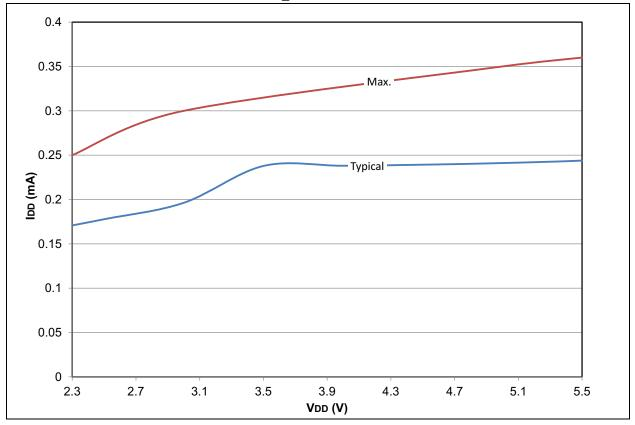
FIGURE 28-26: PIC18LF2X/4XK22 TYPICAL IDD: RC\_RUN HF-INTOSC
