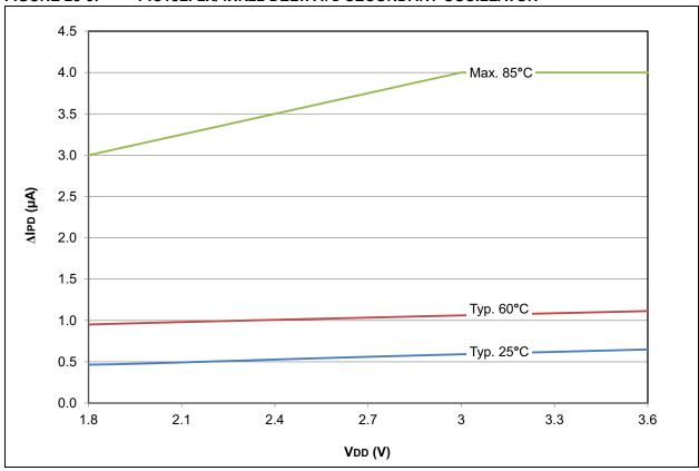
FIGURE 28-10: PIC18F2X/4XK22 DELTA IPD SECONDARY OSCILLATOR
