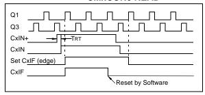
FIGURE 18-4: COMPARATOR INTERRUPT TIMING WITH CMxCON0 READ
