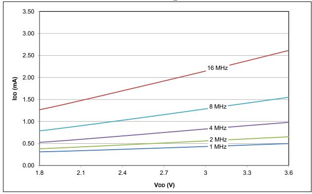
FIGURE 28-27: PIC18LF2X/4XK22 MAXIMUM IDD: RC\_RUN HF-INTOSC
