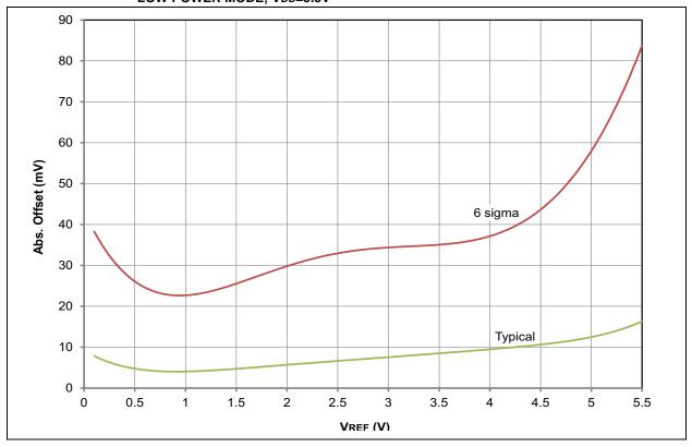
FIGURE 28-91: PIC18(L)F2X/4XK22 COMPARATOR OFFSET VOLTAGE, LOW-POWER MODE; VDD=3.0V
