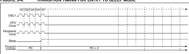
FIGURE 3-4: TRANSITION TIMING FOR ENTRY TO SLEEP MODE
