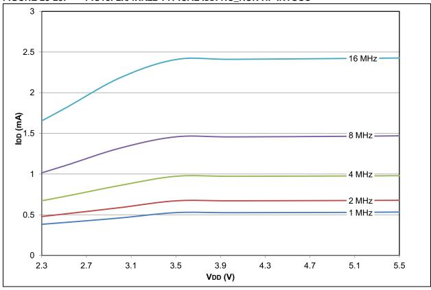
FIGURE 28-29: PIC18F2X/4XK22 MAXIMUM IDD: RC\_RUN HF-INTOSC
