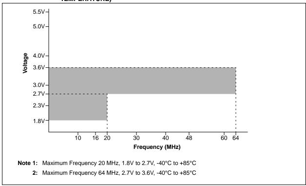
FIGURE 27-2: PIC18LF2X/4XK22 FAMILY VOLTAGE-FREQUENCY GRAPH (EXTENDED TEMPERATURE)
