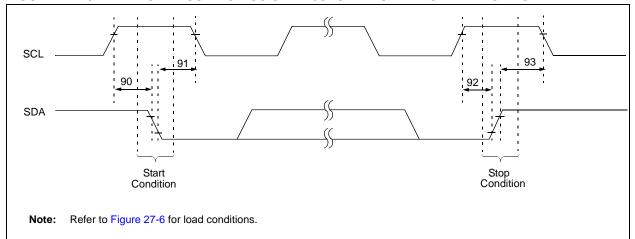
TABLE 27-17: MASTER SSP I<sup>2</sup>C BUS START/STOP BITS REQUIREMENTS
