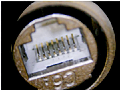
figure 14 – NE8FDX-Y6 after 1000 mating cycles
