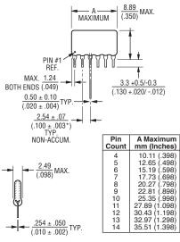
Maximum package length is equal to 2.54mm (.100") times the number of pins, less .005mm (.002")
