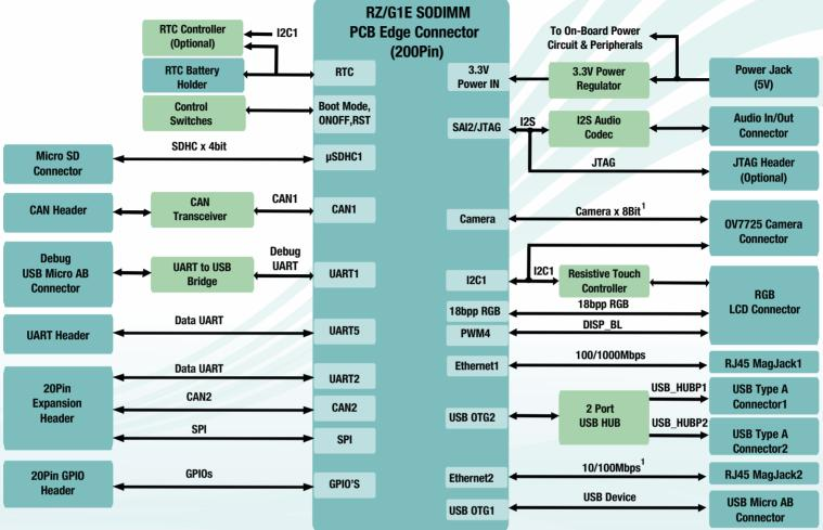
*Note1: 2<sup>nd</sup>Ethernet and 8-bit camera interface is multiplexed in the RZ/G1E CPU. At a time anyone can be used. By default 8-bit camera interface is supported in the development kit.*
