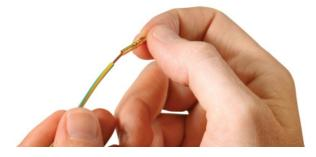
7) To crimp contact assembly-cable, tighten sharply the clip to the end of the mechanism (maxi 175N).
