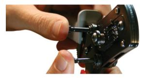
5) Place conductors, with no deteriorations, in the bucket contact. All strands to be located in the crimp bucket.
