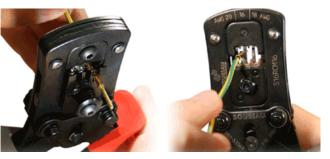
8) To control crimp quality, slighty pull cable with two fingers to control retention.
