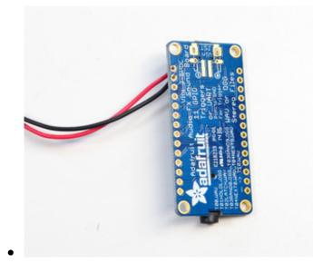
For most battery packs the red wire is the positive wire, connect that to Vin. The black wire is ground, connect that to GND.
