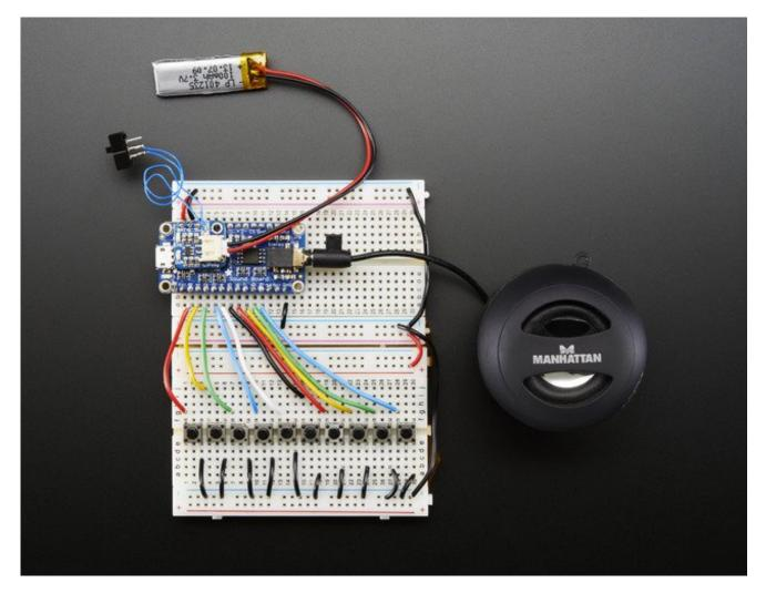
You can see each button connects to the trigger pin, and then the other side to ground. For
