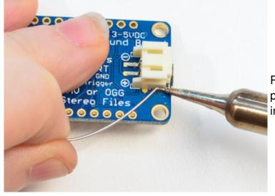
Place the JST and solder that pad onto the connector to tack it in place
