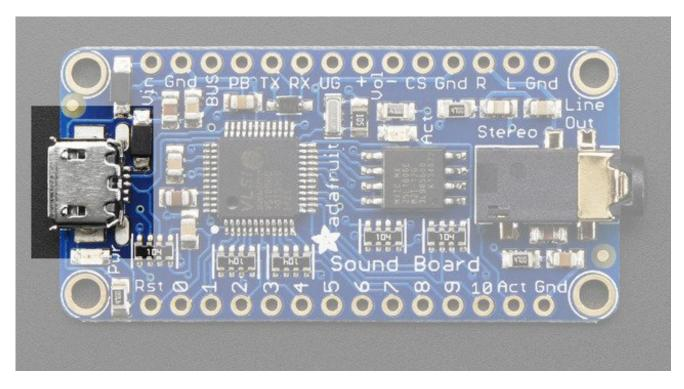
Starting from the left is the micro USB jack. You'll need a standard MicroUSB cable to connect this to your computer. You do need a computer (any will do) in order to save files onto the Sound Board flash storage
