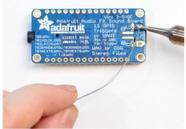
Start by melting some solder onto one of the side pads of the JST footprint on the bottom
