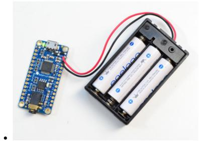
The nicer battery packs have switches, or you can just remove the batteries when not in use. If the green light is lit, it's powered up!
