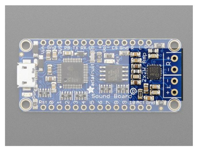
All the way to the right is the Class D stereo amplifier. This is for connecting to a pair of speaker! The outputs are bridge-tied-load (BTL) so do not connect R+ to L+ and R- to L- to get more power, it could damage the chip. If you only need one speaker, simply connect the channel you want.
