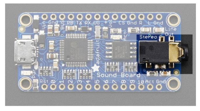
All the way to the right is the headphone jack. This is for connecting to a pair of headphones or into a powered speaker. It cannot drive an 8 ohm or 4 ohm speaker. Instead, an amplifier will have to be used (basically, just like your phone or pocket MP3 player needs an external powered/amplified speaker)
