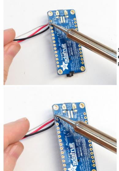
Solder both wires securely. You **cannot** just twist the wires into place!
