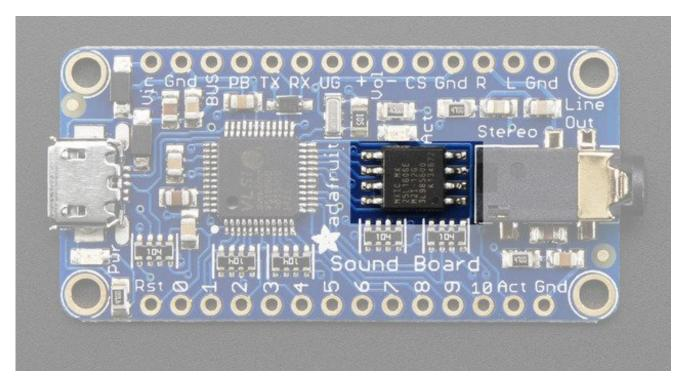
This is the onboard flash chip. It's basically like a little SD card, but soldered directly onto
