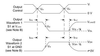
Voltage Waveform Enable and Disable Times
