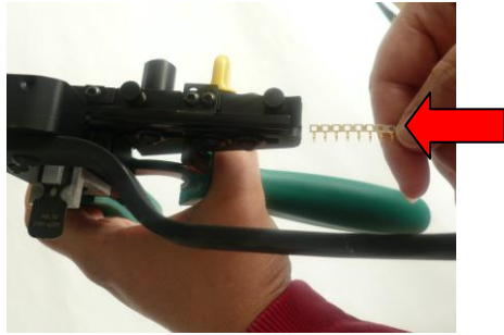
Insert the strip of contacts into the feed unit. Kontaktstreifen in Vorschubeinheit legen.
