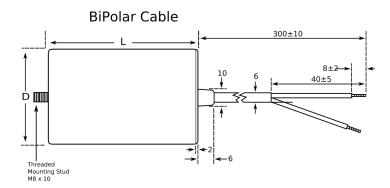
Series C27 Dielectric Film/Foil Polypropylene Style Plastic Case and Cover, Ultra Sonically Welded Description Ultra Sonically Welded Seal, Safety Class PO, **Features** UL 94 V0 Disk RoHS Yes Termination Tin Copper **BiPolar Cables** UL, VDE, UL (Construction Only), UL\_94 VO Disk Qualifications AEC-Q200 Component 156.8 g Weight
