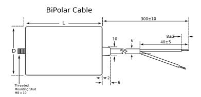
General Information Series C27 Dielectric Film/Foil Polypropylene Style Plastic Case and Cover, Ultra Sonically Welded Description Ultra Sonically Welded Seal, Safety Class PO, **Features** UL 94 V0 Disk RoHS Yes Termination Tin Copper Lead BiPolar Cables UL, VDE, UL (Construction Only), UL\_94 VO Disk Qualifications AEC-Q200 Component 39.08 g Weight
