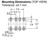
Note 1. Each value has a tolerance of ±0.3 mm. Note 2. The coplanarity of the terminals is 0.1 mm max.
