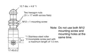
Note: Unless otherwise specified, a tolerance of  $\pm 0.4 \ \text{mm}$  applies to all dimensions.
