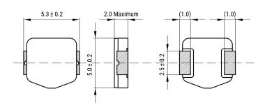
General Information Series MPX Style SMD Chip Size 0520(2120) Description Surface Mount Inductor Features Power Inductors **RoHS** Yes Core Composite Miscellaneous 40 (K) Temperature Rise Max.
