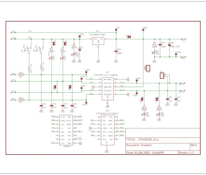
Figure 4 Schematic of ITS42k5D-LD-F Demo board (PG-TSO-10)
