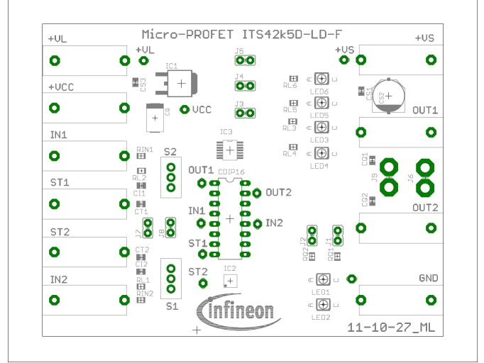
Figure 7 Top Layer components of ITS42k5D-LD-F Demo board (PG-TSON-10)
