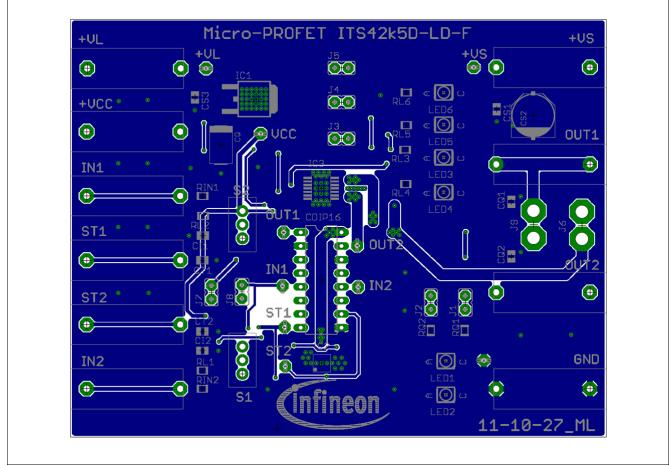
Figure 6 Bottom Layer of ITS42k5D-LD-F Demo board (PG-TSON-10)
