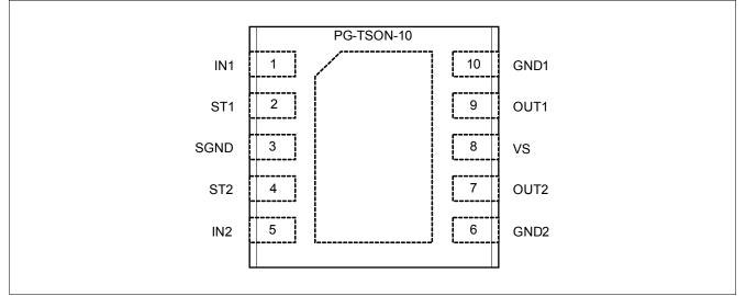
Figure 2 Pin-Out of the ITS42k5D-LD-F
