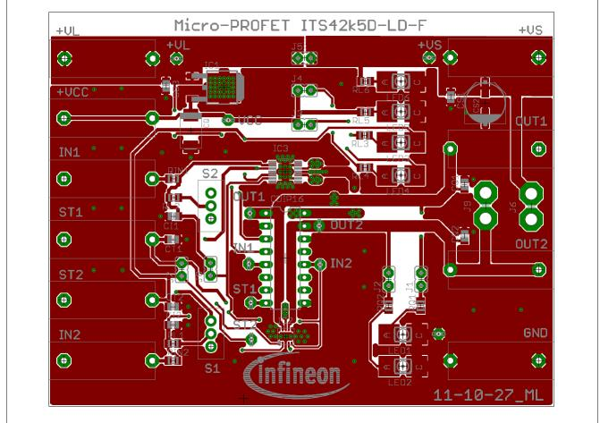
Figure 5 Top Layer of ITS42k5D-LD-F Demo board (PG-TSON-10)
