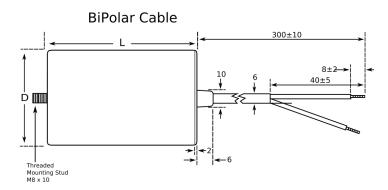
General Information Series C27 Dielectric Film/Foil Polypropylene Style Plastic Case and Cover, Ultra Sonically Welded Description Ultra Sonically Welded Seal, Safety Class PO, UL\_94 VO Disk **Features** RoHS Yes Termination Tin Copper Lead BiPolar Cables UL, VDE, UL (Construction Only), UL\_94 VO Disk Qualifications AEC-Q200 Component 97.86 q Weight
